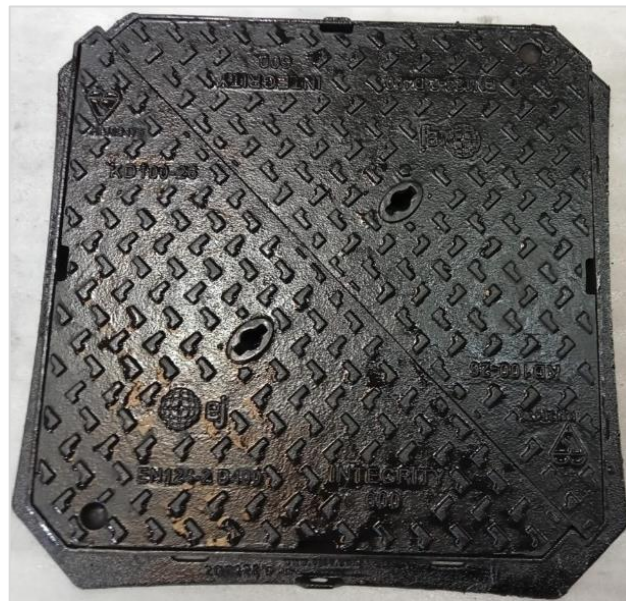
KD100-26E (600X600X100 DOUBLE TRIANGULAR D400 FRAME AND COVER), 61 KG, DUCTILE IRON EN 1563 GRADE 500/7
