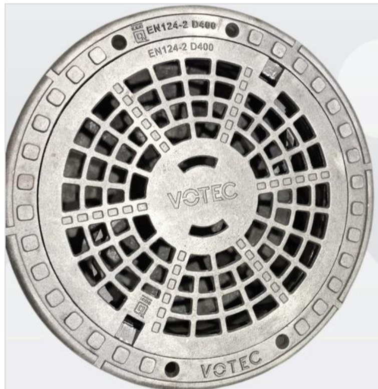
600 DIA X 190 D400 SELF LOCK GRATE AND FRAME - WEIGHT 84 KG
