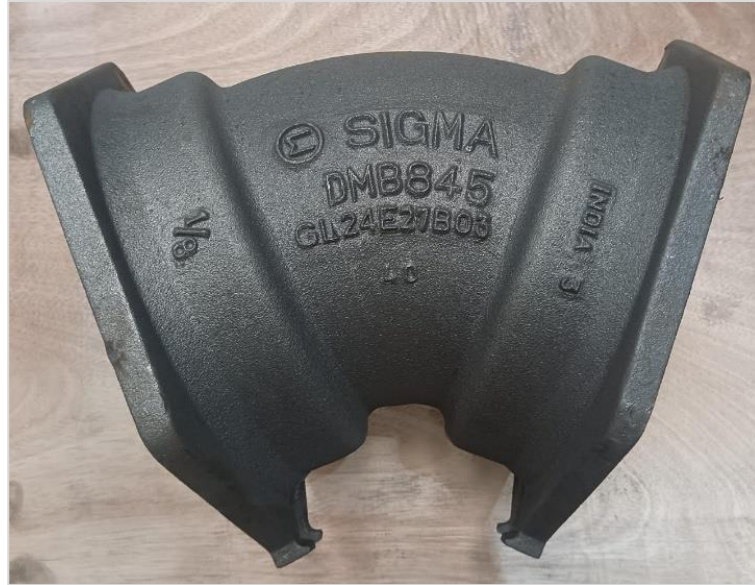
DMB845 (8 " AND 45 ° BEND, 20.87 KG), DUCTILE IRON ASTM 536 GARDE 70-50-5
