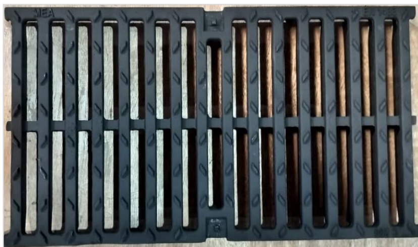
GRATE 010712846 C250 498X222, 6.2 KG, DUCTILE IRON EN 1563 GRADE 500/7
