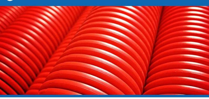
GrainDuct cable protection pipe is produced from PE in diameters Ø 40mm, 50mm, 63mm, 75mm, 90mm, 110mm, 125mm, 160mm and 200mm, on flexible coils of 25 meters or 50 meters and on rigid 6 meter lengths, all fitted with click-sockets.
